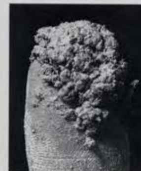
FIG 10A Sandy loam: a ribbon less than 2.5 cm long forms; individual grains are visible.
