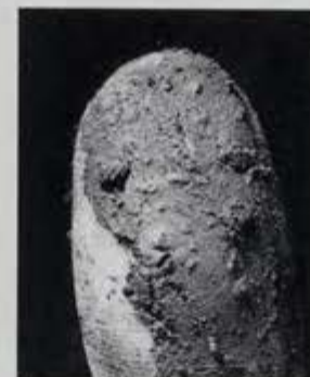
FIG 10B Clay loam: a ribbon 2.5 to 5 cm will form; soil appears smoother.
