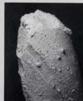
FIG 10C Clay: a ribbon greater than 5 cm can be formed; soil glistens somewhat.
